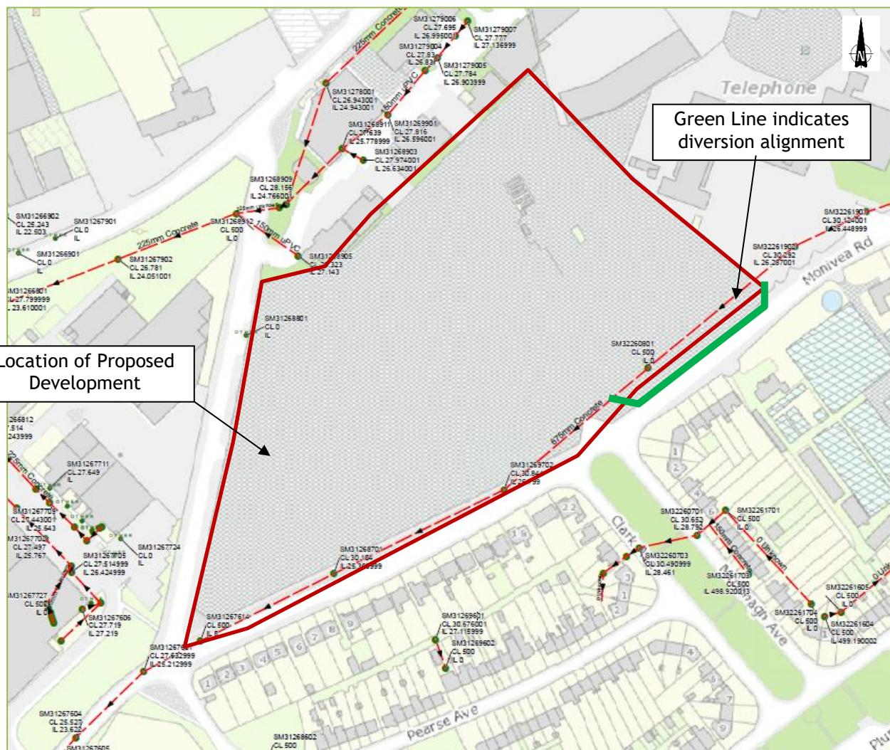
Figure 2 - Existing Foul Drainage Surrounding Site (Source: Irish Water Record Drawing)
